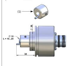
Please mount the encoder into the easy-clamp-flange. The cylinder bolt must slip into the spring (2).
